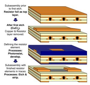
**Figure 2: Processes for Defining Resistor Elements**
