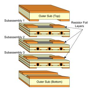
Figure 1: Stack up of multilayer PCB with subassemblies and multiple embedded resistor layers.
